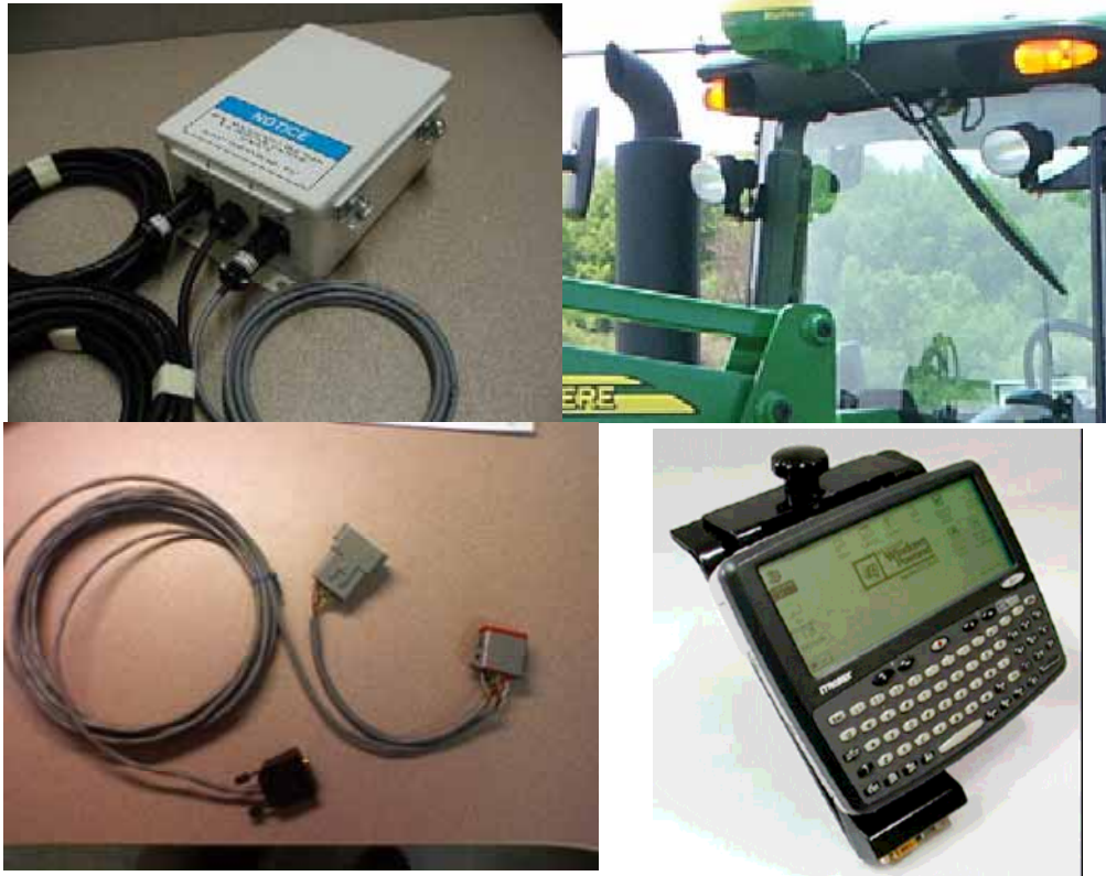
Figure 1. Components of the SkyTrip system that triggers the planter.
