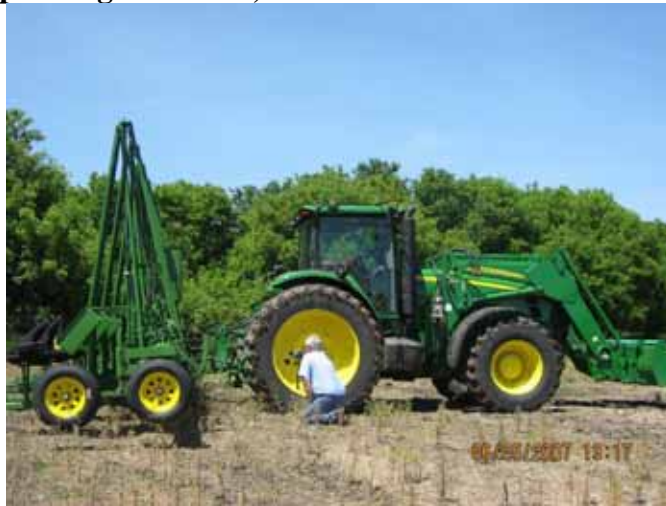
Figure 6. Planter weight is balanced by front-end loader on tractor.
