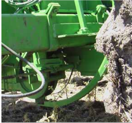
Figure 5. Curved skid attached to bottom of injection slot. Mud on tractor tires shows field was too wet for planting on June 5, 2007.
